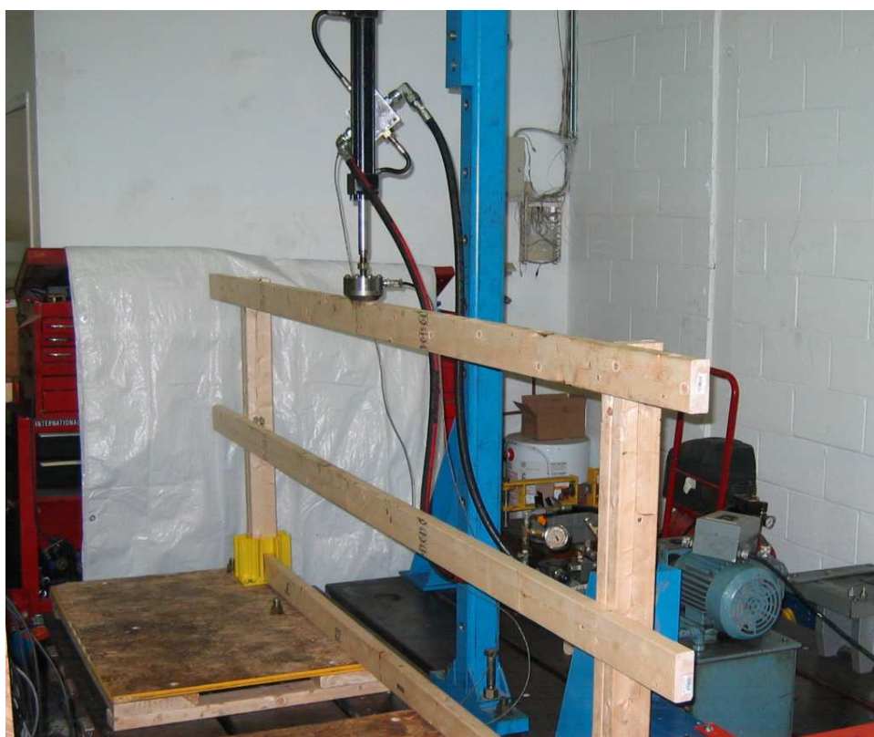
Figure 4: Top rail vertical load test
